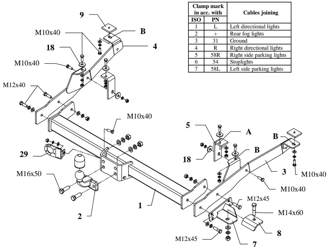
This towing hitch is designed to assembly in following cars: **FIAT DUCATO, PEUGEOT BOXER, CITROEN JUMPER, 2WD and 4WD, metal build-up, loading platform**, produced since 05.1994 till 06.1999, catalogue number **R08** and is prepared to tow trailers max total weight **2000 kg** and max vertical load **100 kg**.
